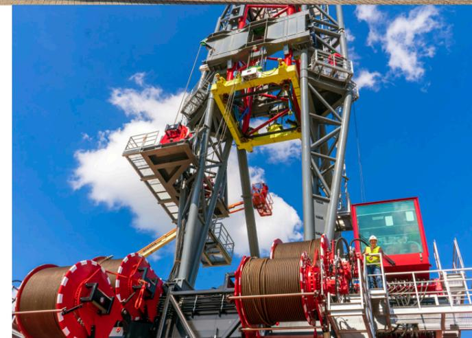
variable superlift system and also a variable superlift tray. This allows the FOCUS30 to take on multiple lifts of different weights and at different radii without reconfiguration or changing the ballast. This means fewer interruptions to work on site, and greater efficiency.
