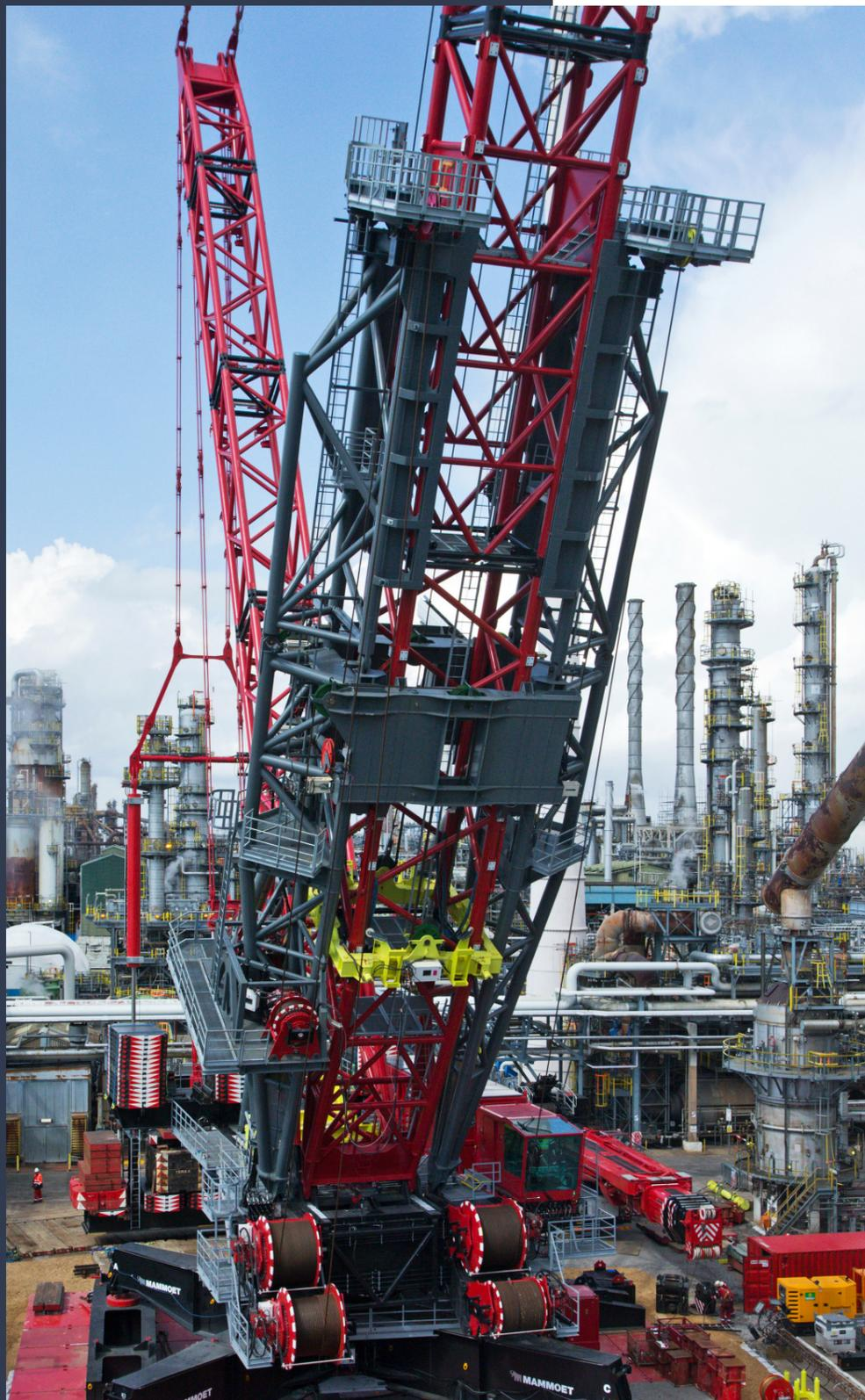
**T**he innovative FOCUS30 crane helped to reduce disruption during scheduled turnaround activity at a refinery in the UK. The crane performed a top-and-tail lifting operation in tandem with a 500-tonne mobile crane, in order to install a vessel at the facility.
